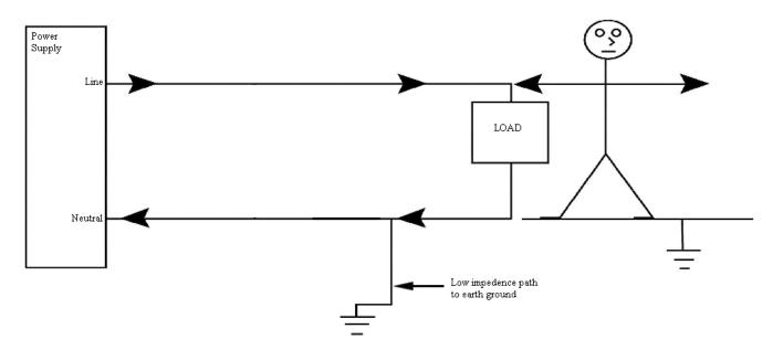
Figure 4: Distribution system with neutral tied directly to earth ground. This provides a low impedance path to earth so in the event of a fault at the load, the person is not the path to ground.
