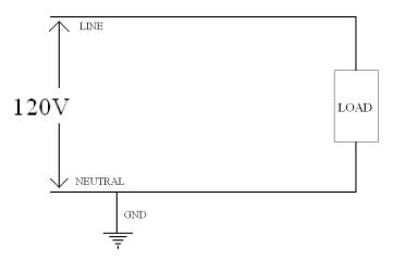
Figure 1: Voltage measurement between line (high) and neutral (low) with the neutral tied to a ground reference point.
