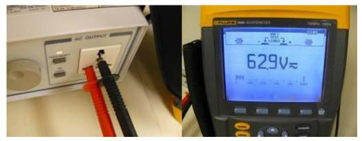
Figure 6d: Voltage measurement between line and ground
