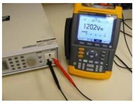
Figure 6b: Voltage measurement of 120.2VAC between line and neutral output
