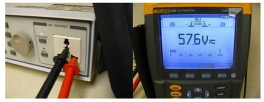
Figure 6c: Voltage measurement between neutral and ground
