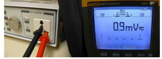
Figure 6c: Voltage measurement between neutral and ground with neutral tied to ground reference.
