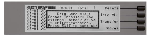
The above message appears when the USB Flash memory drive is write-protected. There are two ways to configure the memory drive as write-protected. One is to set the switch on the side of the memory drive up (towards the drive's connector). The other is to configure it through the drive's properties in Windows.
