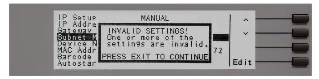
Press the EXIT key to save the new settings. If the IP Setup parameter is set to AUTO, you do not need to enter an IP Address manually.
