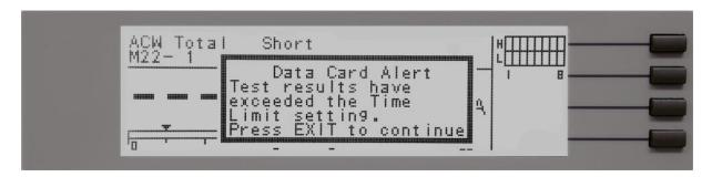
By pressing the EXIT soft key, the message will be cleared and it won't appear again until the unit is re-booted or the Time Limit setting is set to a different value.
