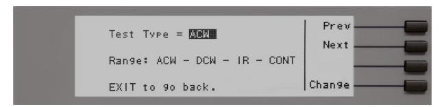
If the selected parameter is a toggle selection, as shown in the example above, the bottom soft key will have the word "Change" next to it. After the "Change" soft key is pressed, the parameter will toggle and you will be prompted to press ENTER to save or EXIT to cancel the edit.
