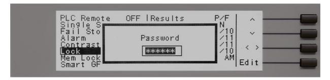
In order for you to access the Lock or Mem Lock parameters, you will now have to enter the proper password. If you have forgotten the password, please refer to the **Forgotten Password** instructions in the Security section.
