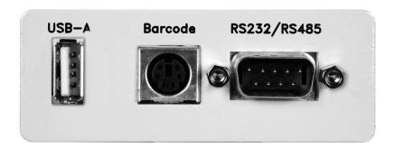
The USB-A port is used for the connection of the USB Flash memory drive.
