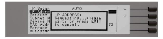
NOTE: The "Requesting IP Address..." pop-up message only appears at power up when the Ethernet Card has its IP Setup configured to AUTO.
