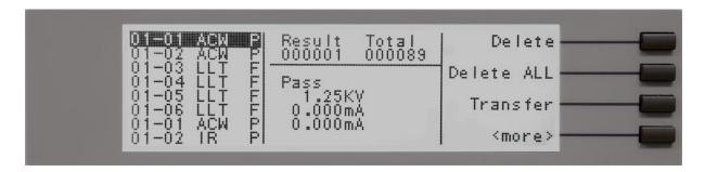
From this menu, the user can view the stored results, delete results, and transfer the results to the external USB Flash memory drive.
