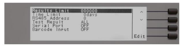
To navigate to the Data Card Settings menu, select the <more> soft key from the Perform Tests screen. Then select the "DCard" soft key. A brief description of the settings follows:
