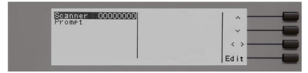
The second or <more> screen will only appear if there is a scanner selection in the menu. The Scanner selections will only appear if there is a scanner installed or an external Scanner connected to the instrument (this is an auto-detect feature in hardware).
