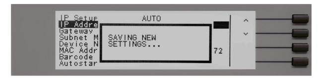
The Ethernet Card will attempt to re-establish a connection with the server anytime the user modifies a parameter and exits the Ethernet Card Parameters Menu or uses the command set at the end of this option description. Thus, if the IP Setup is set to AUTO, the Ethernet Card will request a new IP Address every time a parameter is edited and, as a result, the "Requesting IP Address. . ." message will appear.
