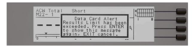
The message gives two options: Pressing Enter will clear the message and display it again at the end of the next test file execution. Pressing Exit will clear the message and not display it again unless the unit is re-booted, or the user deletes all previous results and the total results are exceeded once more.
