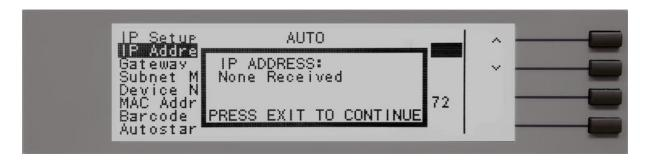
Press the EXIT key to remove the pop-up message and return to the HypotULTRA III's Perform Tests screen.
