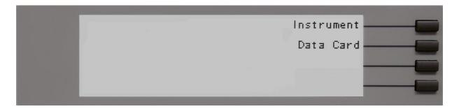
Pressing the "Instrument" soft key will display the detailed results from the previously executed test. Pressing the "Data Card" soft key will display the Data Storage Card Results menu as shown below:
