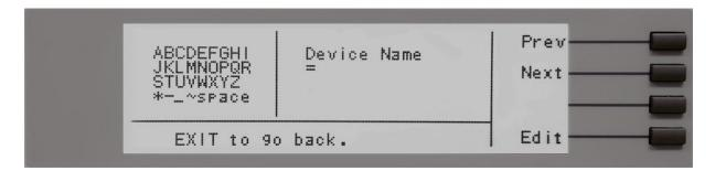
From this screen you may enter a Device Name for the HypotULTRA III. The Device Name is used to identify the HypotULTRA III on your server and may be used in place of a dedicated IP Address. Use the arrow keys to highlight a letter and press the "Select" soft key to select the highlighted letter. The Device Name may be a maximum of eight characters and MUST start with a letter. If the Device Name does not start with a letter the following error message will be displayed:
