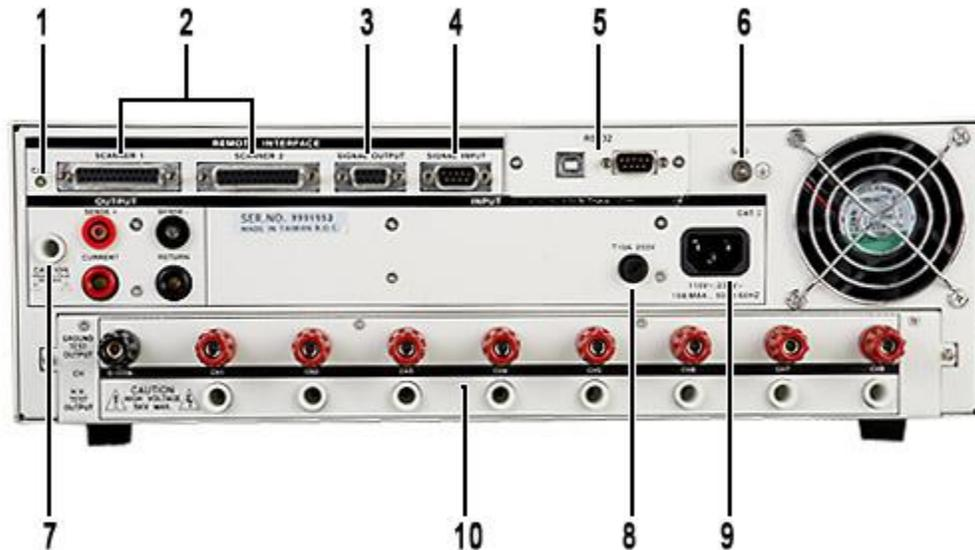
1. **CALIBRATION BUTTON:** To put the instrument into the calibration mode push this button and turn on the power switch simultaneously.
