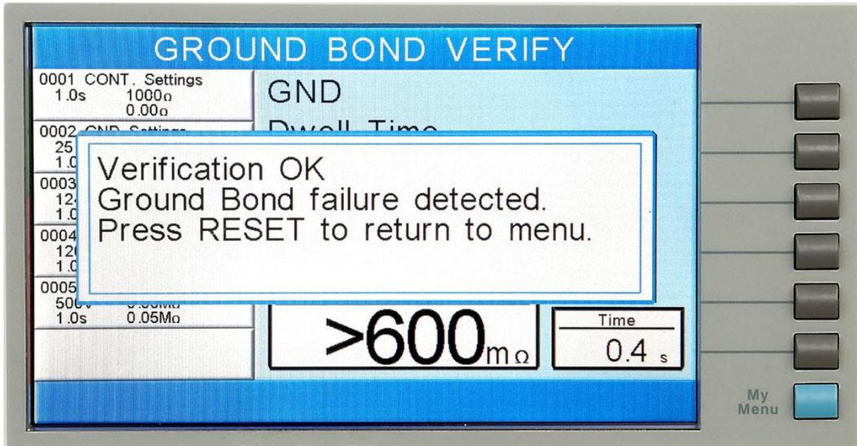
If the instrument fails the Verification (test pass, indicating the fail detectors are not working properly) the TEST button will illuminate and the following pop-up message will appear over the metering screen:
