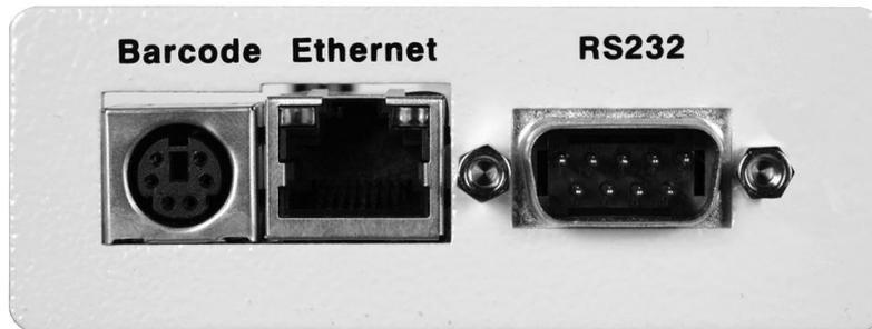
The port labeled “Barcode” is a PS/2-type connector that is used for the connection of a barcode scanner. The Ethernet port is for use with a standard CAT-5 Ethernet cable and may be connected to any compatible PC. The 9-pin D-type subminiature connector labeled “RS232” is for connection of the OMNIA to an RS-232 communication bus.
