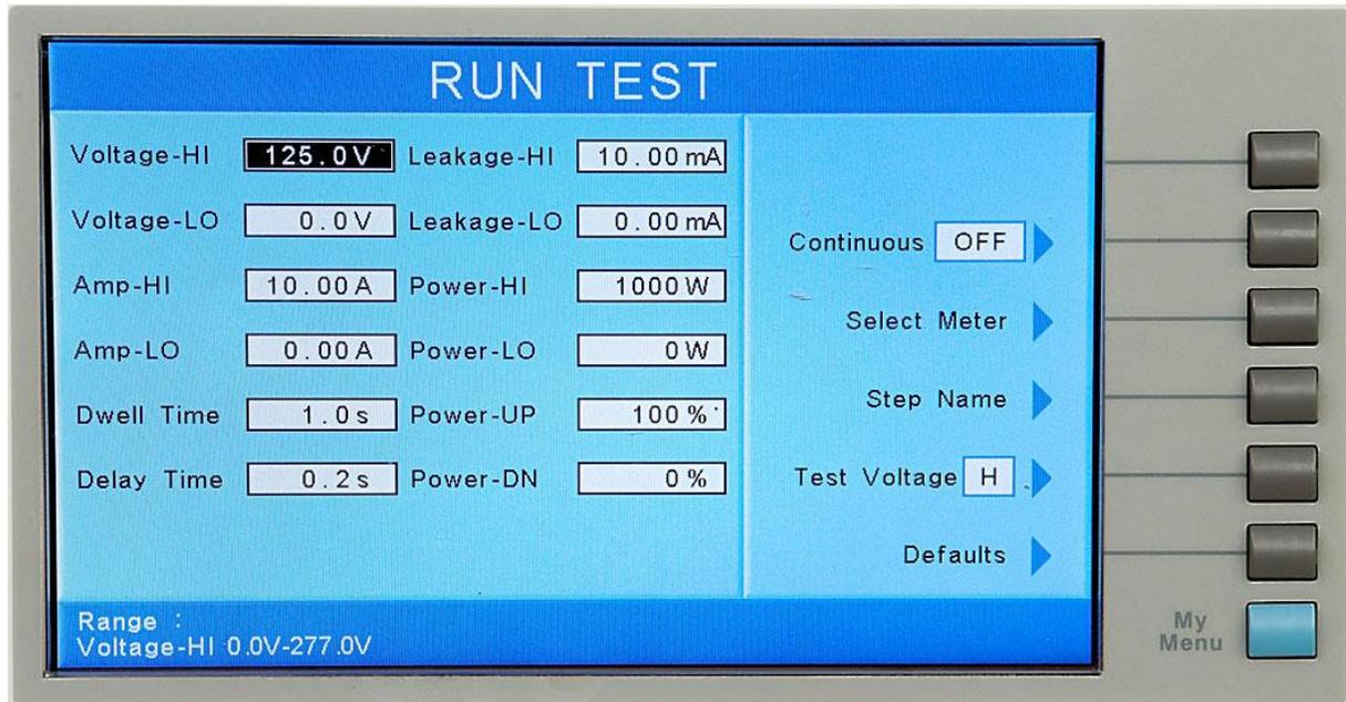
Setting the Test Voltage selection to N, L, and H will create different digital states at Bit 0 and Bit 1 of the PLC Remote Signal Output (refer to the PLC Signal Output drawing below). The different states are described in the truth table below. The “Not used” state is undefined and cannot be programmed for use.
