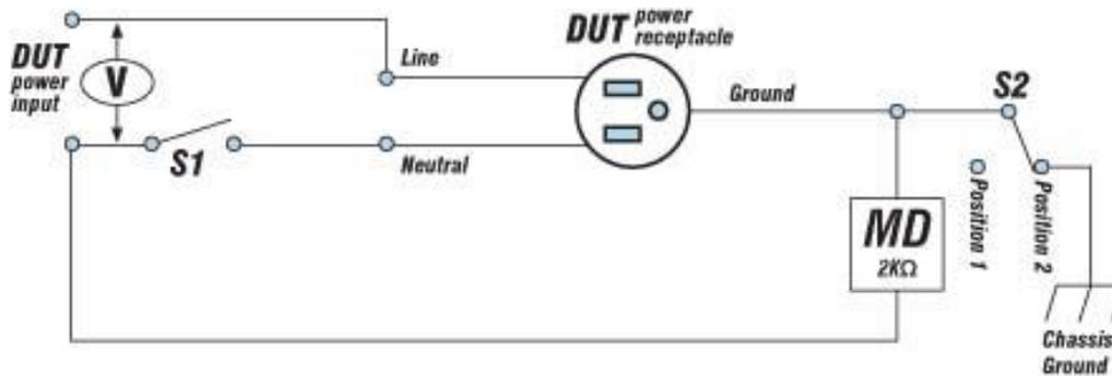
When the Leakage-HI trip limit is set to 0, S2 is placed in position 2 which disables the earth leakage test and connects the neutral of the DUT input to the ground of the DUT.
