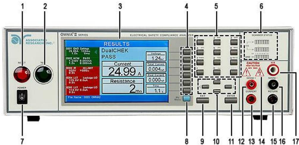
1. **RESET BUTTON:** Resets the instrument. If a failure condition occurs during a test, pressing this button will reset the system, shut off the alarm and clear the failure condition. The Reset button must be pressed before performing another test or changing any of the setup parameters. This button also serves as an abort signal to stop any test in progress.
