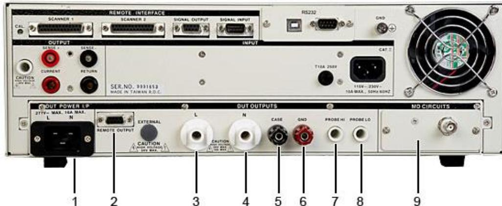
1. **DUT POWER INPUT CONNECTOR:** This connector provides the Line and Neutral input power connections on pin 1 and 2 respectively. An external single phase unbalanced AC power supply with a single Hot or Line conductor should be connected here to supply power to the DUT while performing the leakage test. This input is rated for 0-277 volts 50/60 Hz.
