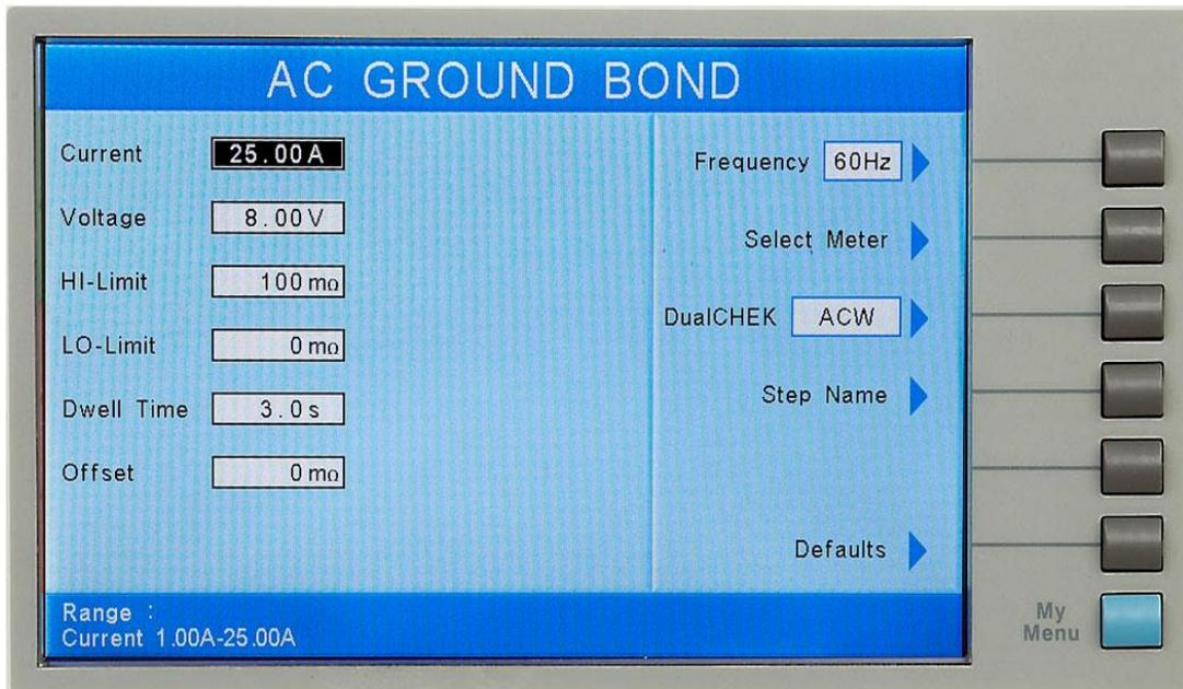
From the Ground Bond Parameter Setting screen, the following parameters may be controlled: Current, Voltage, HI-Limit, LO- Limit, Dwell Time, Offset, Scanner Channel, Frequency, DualCHEK, Step Name and Defaults.
