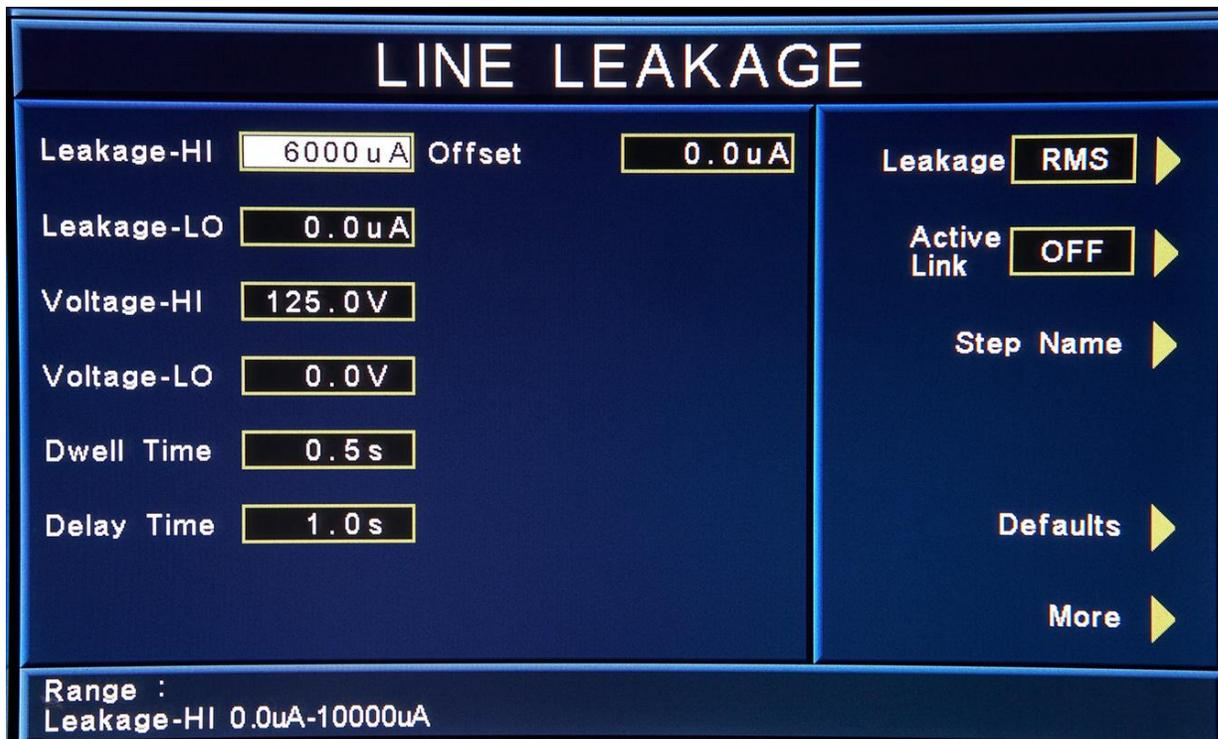
From the Leakage Current Parameter setting screen, the following parameters may be controlled: Leakage-HI, Leakage-LO, Voltage-HI, Voltage-LO, Dwell Time, Delay Time, Offset, Leakage, Active Link, Step Name, Scanner Channel, Defaults and More. Pressing the More key will bring up additional parameters: Reverse, Neutral, Ground, Measuring Device and Probe. Pressing the More soft key again will bring up additional parameters: AC Source, AC/DC, Select Meter, and Ranging Mode.
