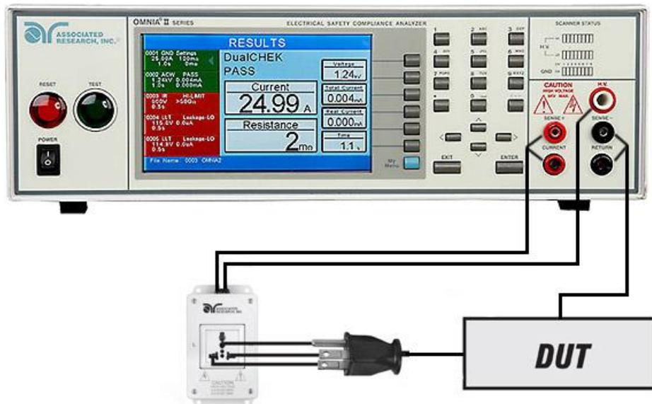
The rear output connections may be used for connecting the adapter box as well.
