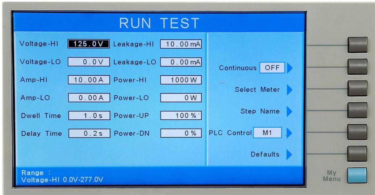
When the Power Tracking and Continuous Output options are installed, the DUT will be connected to the power source during and between test steps. If the power reading increases above the Power-UP percentage or drops below the Power-DN percentage from the previous step, then the next step will begin.
