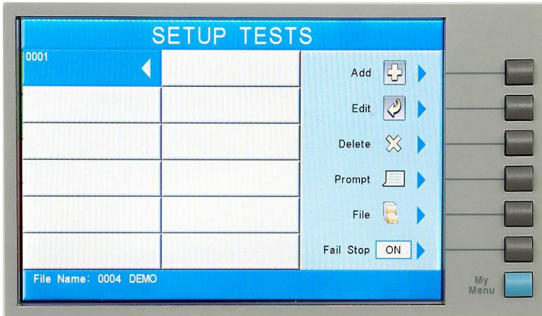
The Setup Tests screen is the central starting point for programming tests into the instrument. From this screen, test parameters are entered and edited, and the order of the test steps can be arranged and then stored to test files. The OMNIA is capable of performing a 10,000-step sequential test from a single test file.
