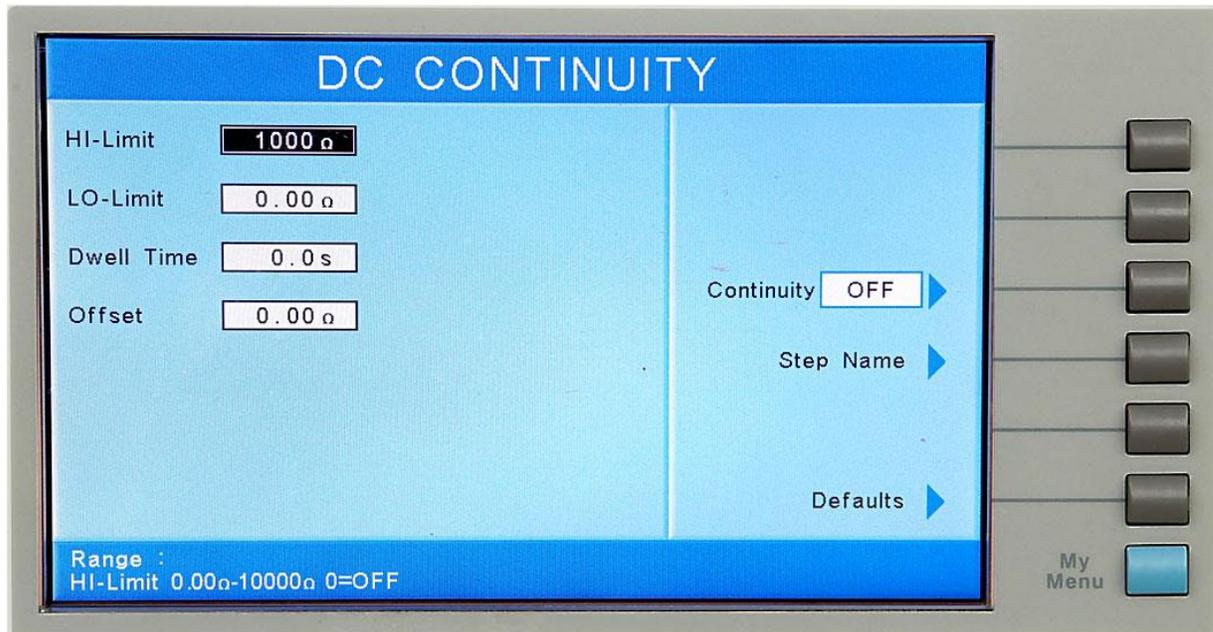
The “Continuity” selection is short for continuity connection and refers to which connection points may be utilized for the continuity measurement. The new continuity parameter has three toggle selections MAINS, GND, and OFF.
