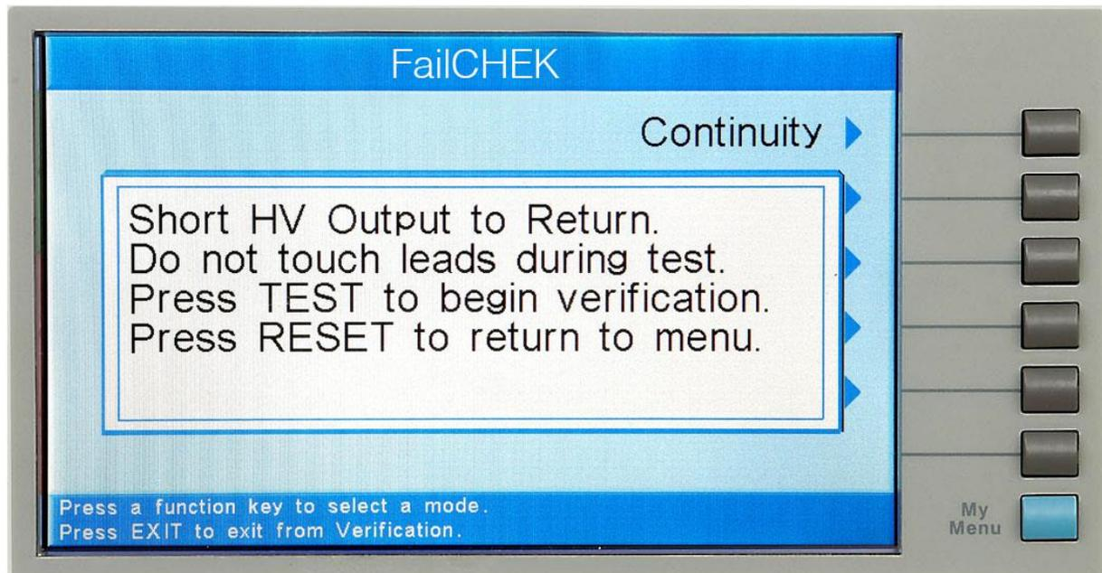
Follow the instructions given in the pop-up message and then press TEST to begin the verification process. During the Verification process the metering screen for the related process will be displayed, refer to section **5.4. Perform Tests Metering** for more information.
