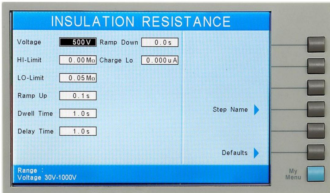
From the Insulation Resistance Parameter Setting screen the following parameters may be controlled: Voltage, HI-Limit, LO- Limit, Ramp Up, Dwell Time, Delay Time, Ramp Down, Charge-LO, Scanner Channel, Select Name and Defaults.
