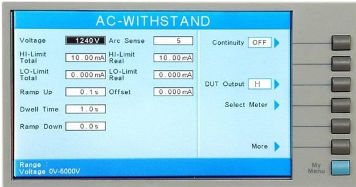
This provides additional settings to control the DUT Output L and N terminals during ACW, DCW and IR tests. When this option is installed and the DUT-HV setting is enabled in the Setup System screen an additional parameter will be available in the ACW, DCW and IR Test Parameter Settings screen. The operator can configure the DUT Output L and N terminals to O (off), H (which places them at high potential) or L (which places them at return potential). Refer to the table below for more details.
