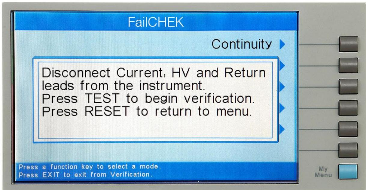
Follow the instructions given in the pop-up message and then press TEST to begin the verification process. During the Verification process the metering screen for the related process will be displayed, refer to section 5.4. **Perform Tests Metering for**
