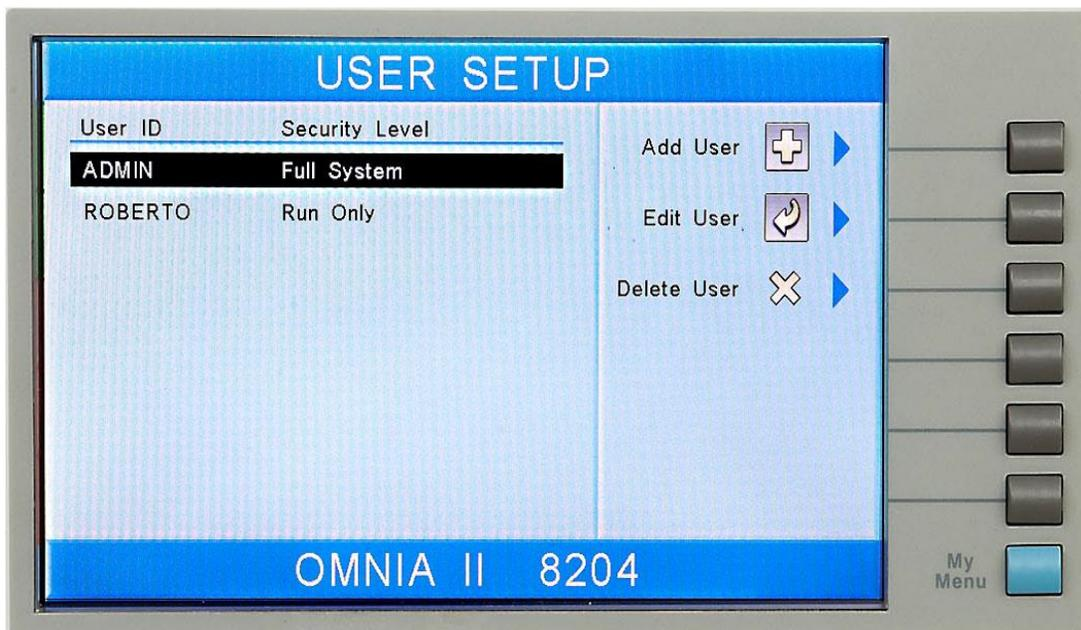
From the User Setup screen, you can view the list of users currently setup and the associated security level. The OMNIA will have a default User ID named ADMIN with Full System Access security level. This User ID cannot be deleted.
