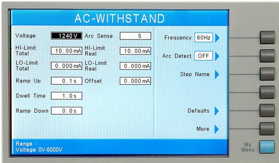
From the AC Withstand Parameter Setting screen the following parameters may be controlled: Voltage, HI-Limit Total, LO-Limit Total, Ramp Up, Dwell Time, Ramp Down, Arc Sense, HI-Limit Real, LO-Limit Real, Offset, Frequency, Arc Detect (ON/OFF), Step Name, Scanner Channel, Defaults and More. Pressing the More soft key will display the additional parameters Continuity selection (DC continuity or OFF) and Select Meter.
