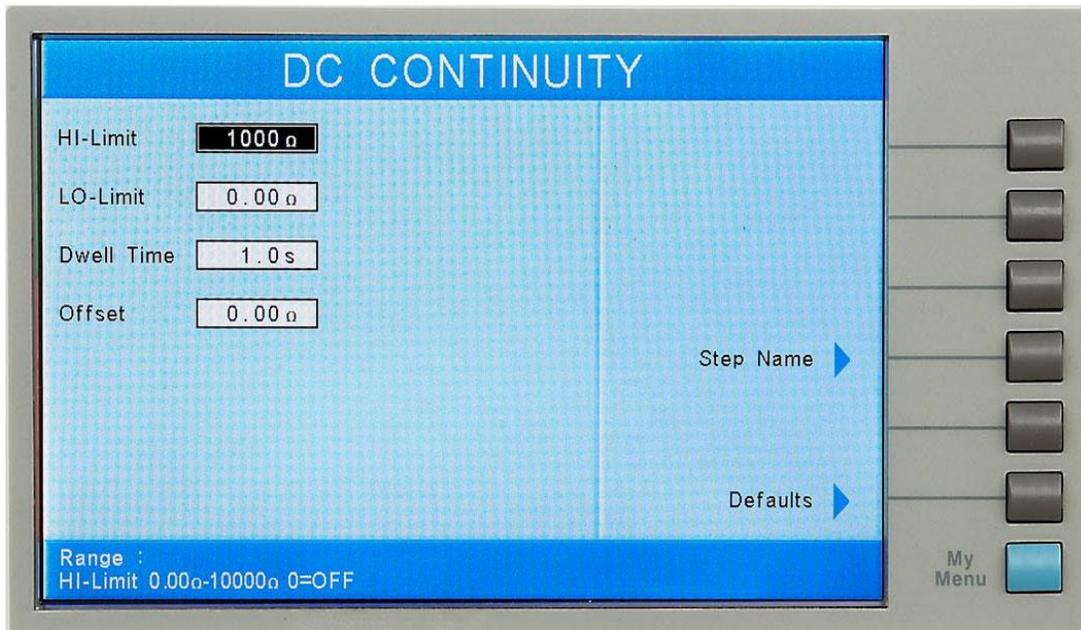
From the Continuity Parameter Setting screen, the following parameters may be controlled: HI-Limit, LO- Limit, Dwell Time, Offset, Scanner Channel, Step Name and Defaults.
