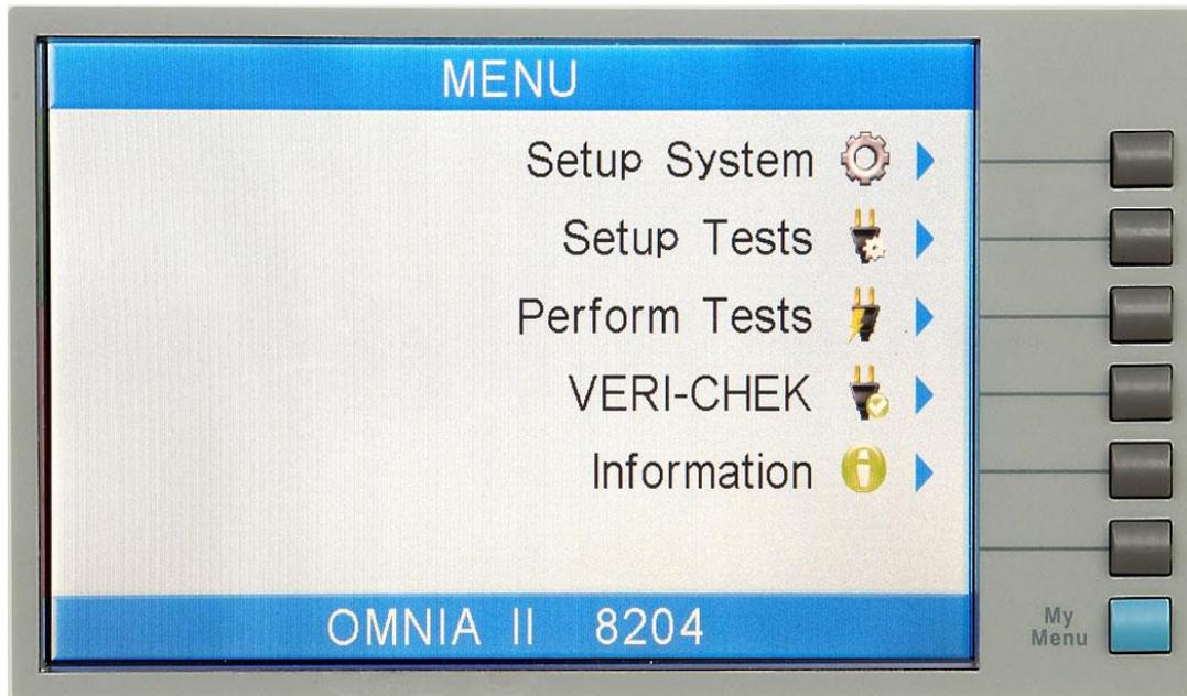
From the Main Menu screen five menus screens may be accessed: Setup System, Setup Tests, Perform Tests, FailCHEK and Information
