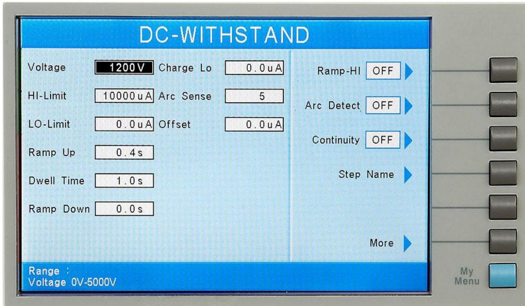
From the DC Withstand Parameter Setting screen the following parameters may be controlled: Voltage, HI-Limit, LO-Limit, Ramp Up, Dwell Time, Ramp Down, Charge-LO, Arc Sense, Offset, Ramp-HI (ON/OFF), Arc Detect (ON/OFF), Continuity (DC continuity or OFF), Scanner Channel, Step Name and More. Pressing the More soft key will display the additional parameter Defaults.
