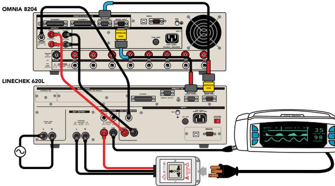
1. Plug the double sided interlocks (P/N 38142) into the signal inputs of both instruments.
