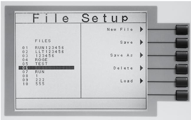
Using the up and down arrow keys, highlight the number of the file slot where the test sequence is to be saved. Hit the "Save As" soft key and the Create File screen will appear.
