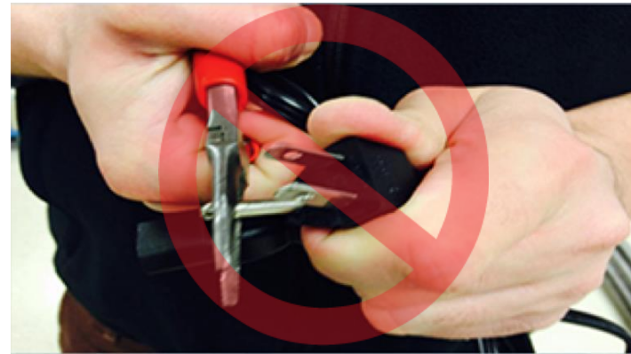
Breaking Ground Pin On Test Equipment
