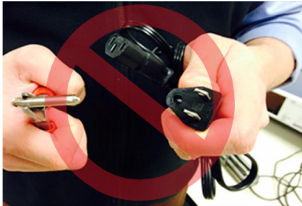
Broken Ground Pin
