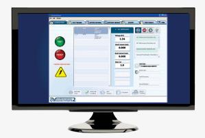
The program also has the capability to associate a product's model and serial number with a particular test sequence. When the model and/or serial number is entered by the operator, the proper test sequence automatically loads. Also, text, audio and video instruction prompts can be added to each step of the test sequence. This allows detailed instructions to be added to each test. This negates user error in running an incorrect test sequence.
