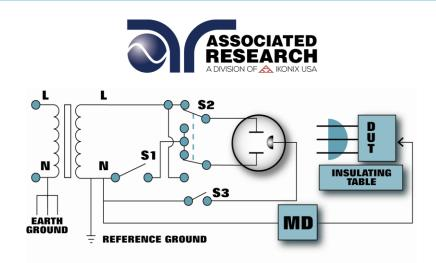
Figure 3: Enclosure Leakage Test Isolated Input, The Output of the Isolation Transformer is not Referenced to Earth Ground
