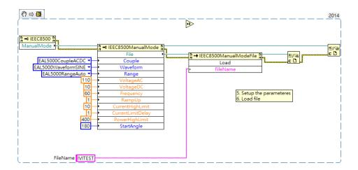
For the EEC8500, all of the test parameters would be within a file. Therefore, you need to create a file first and then select a file to be edited. Also, there are many differences between Standard and Advanced levels of EEC8500. In this example, the configurations of *CoupleACDC*, *Waveform* are not available in the Standard level of EEC8500.
