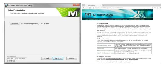
Please download the latest IVI Shared Components either 32-bit or 64-bit version. After downloading, install the shared components and continue the installation.
