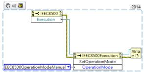
Before we create a Manual Mode file on the EEC8500 power supply, we have to switch the operation mode to Manual Mode. The SetOperationMode() method is under the Execution interface. Please be noted that only the Advanced level of 8500 supports the Step, Pulse and Library modes.
