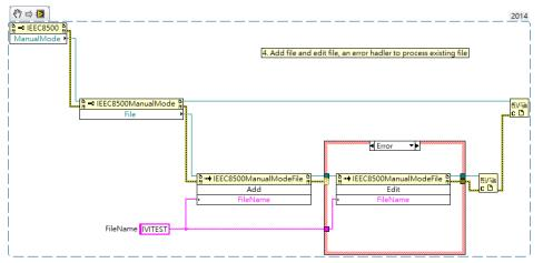
Use the **Property Node** to get reference of the sub-system of **IEEC8500** class. For example, **File** is one of the sub class of **IEEC8500.ManualMode**, and then we could use the **Add** method under **File** to create a file in the device.
