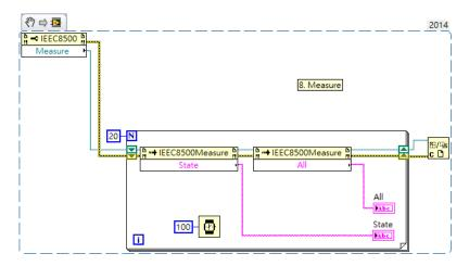
This for loop would run with polling the state and meters. Using the methods of Measure subsystem could let you read the immediate readings.
