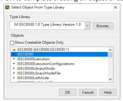
The Labview will automatically generate an *Automation refnum* of *EEC8500Lib.IEEC8500* control and connect to the Automation Open function.
