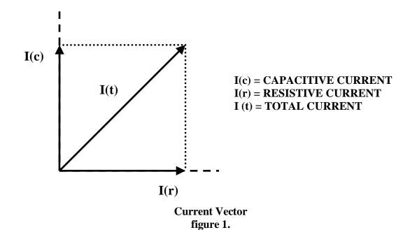
The capacitive leakage is an inherent characteristic of the device controlled primarily by design details. The resistive leakage is a characteristic of insulating materials used and the amount of resistive leakage is generally an indication of the quality of the insulation. This is particularly true when identical devices are being comparatively tested. Both capacitive and resistive leakages vary, almost linearly, with the applied test voltage.
