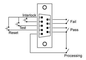
Pins 1 and 6 provide the PROCESSING signal.
