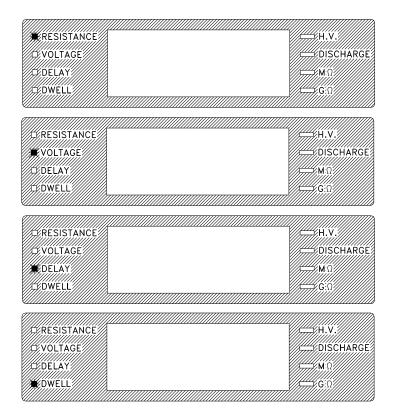
Total cycle time is the delay time plus the dwell time. At the completion of the dwell time, the instrument will 'chirp' to signal the operator that the test cycle has been completed.
