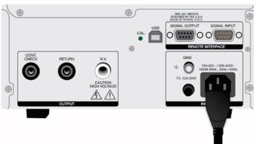
**Step 3** - Connect male end of E-Stop to input power.
